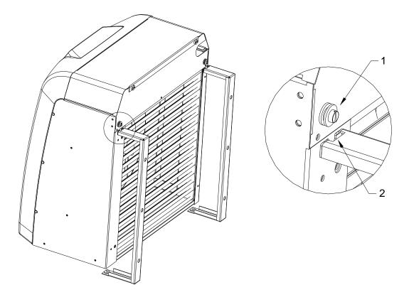
• Position the outside unit so that the screws and washers 1 are engaged in the slot 2
