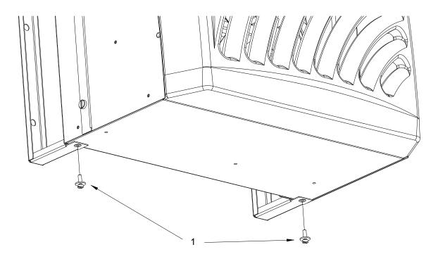
• To finish, screw the kit screws and washer 1 under the unit.
